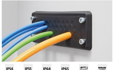
The KEL-DPR 24 cable entry plate is based on the proven KEL-DP 24, but has an integrated polypropylene reinforcement frame. With the KEL-DPR 24, up to 48 cables from 1 to 16.1 mm can be inserted in the smallest of spaces and sealed in accordance with IP65.
