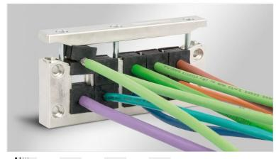
The EMC cable entry frames EMC-KEL-U are based on the KEL-U and KEL-E. Due to a conductive surface, disturbances in the cable shields on the control cabinet can be easily dissipated. Field bound disturbances are derived by the metallisation.
