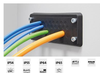
The KEL-DPR 24 cable entry plate is based on the proven KEL-DP 24, but has an integrated polypropylene reinforcement frame. With the KEL-DPR 24, up to 48 cables from 1 to 16.1 mm can be inserted in the smallest of spaces and sealed in accordance with IP65.
